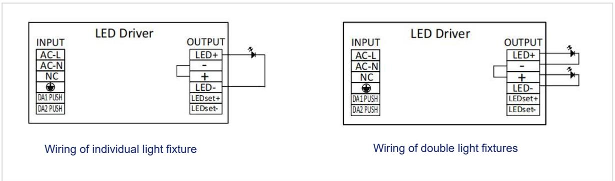
**⚠** Do NOT connect LED set+ to LED- in case of the damage of LED driver.
